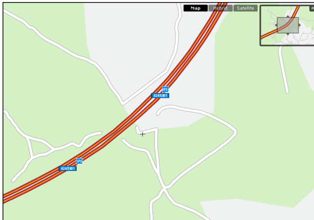
Figure 5.3: Generalization by aggregation. Two roads that are almost parallel are represented as two separate elements in the map, but in the overview map of the upper-left corner, with a smaller level of detail, they are generalized as one single element. (Taken from Yahoo Maps.)
